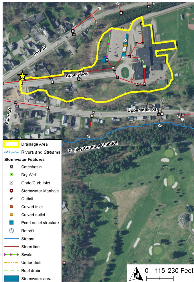
Figure 10. The BMP drainage area is shown in yellow for the Copley Park site. The proposed BMP location is shown with a star.
